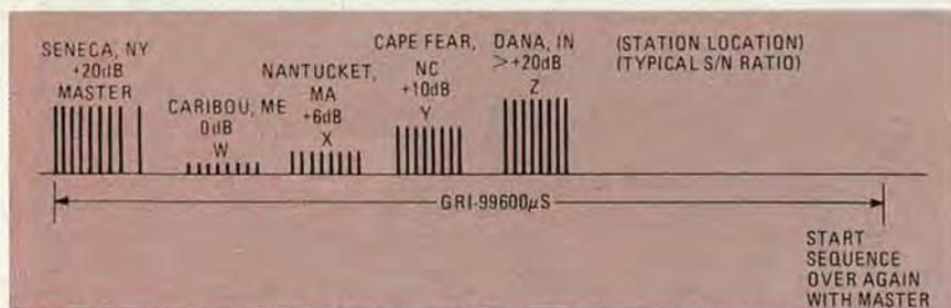
FIG. 4—RELATIVE ENVELOPE AMPLITUDES of a Loran-C chain as received in the midwestern US. Note the "extra" pulse that identifies the master.
