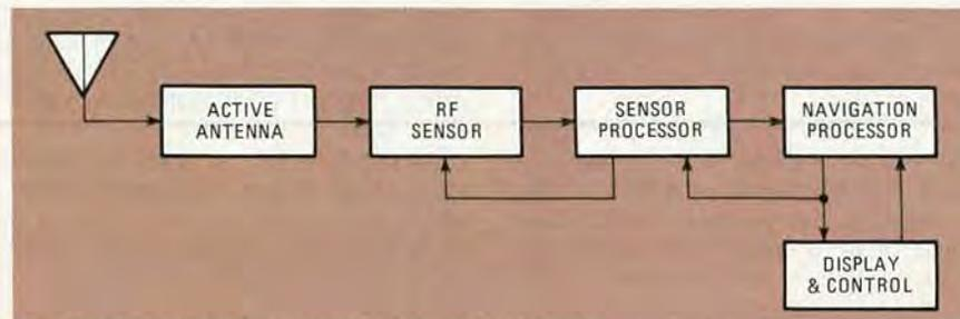
FIG. 2—BLOCK DIAGRAM of a Loran-C navigation receiver.
